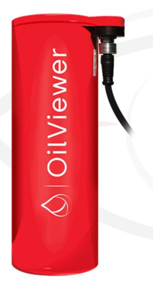
Specifically designed for real time detection of oil spills on water and ground surfaces in continuous automatic mode. It detects the specific fluorescence of oil caused by its exposure to certain UV light emissions, while not reacting to other materials that may appear in the observation area, in order to reduce false alarms.
