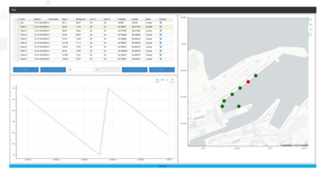
Multiple OilViewer units can be linked together and displayed on a map in your control room. In case of alarms the unit which triggered the alarm is shown in red, as opposite, in order to locate the spill. 04
